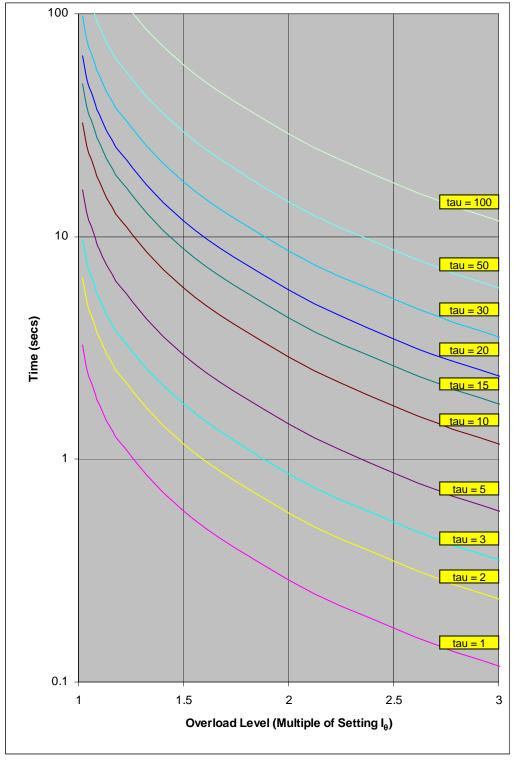
Figure 2 – IEC60255-8 cold curve (tau in seconds)
