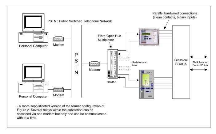
Figure 3 - Star Type Configuration (Using SIGMA-1 Multiplexer)
