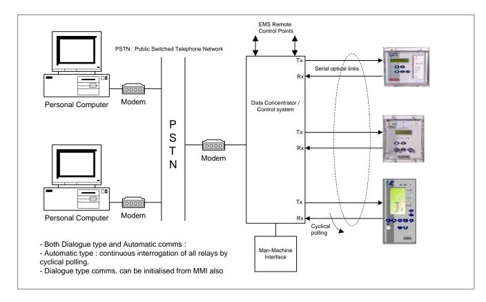
Figure 5 – Direct Control System/Data Concentrator Configuration
