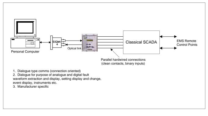
Figure 1 - Basic Communications Configuration
