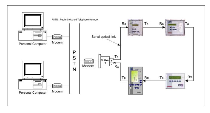
Figure 4 - Optical Ring Configuration (Using SIGMA-4 Fibre/RS232 Convertor)
