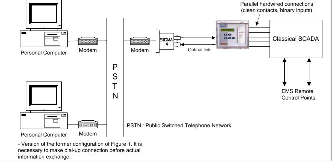
Figure 2 - Basic Communications Configuration (Remote)
